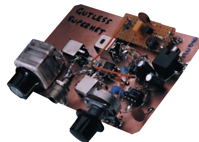
● Heading Photograph The Rev. George Dobbs G3RJV produces a Sudden conversion! However, he's not adding to his congregation - but instead explains how you can change the original Sudden DC receiver into a simple 'Gutless Wonder' superhet.
